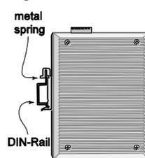
To remove the IE-SW-PL08M switch from the DIN-Rail, simply reverse Steps 1 and 2.
