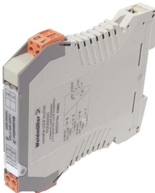
The WavePak Loop Splitter module is a 4-20mA current loop isolator with one loop powered input and two independent, loop powered, isolated outputs. It is ideal for interfacing one transmitter to two devices such as a PLC and a local indicator.
