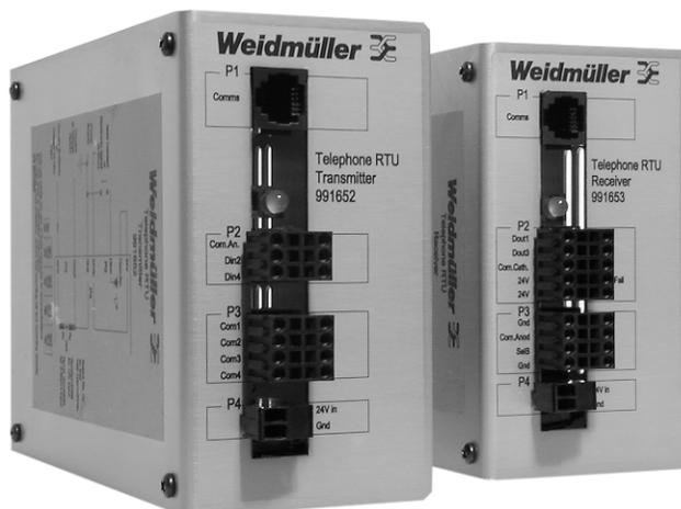
The Telephone RTU system consists of a pair of devices, a transmitter and a receiver that allow the transmission of 4 analog and 4 digital signals over a twisted pair or dedicated telephone line. The signals are encoded and transmitted as a unidirectional FSK signal. The 4 analog input signals at the transmitter are multiplexed to a single analog output at the receiver. There are 2 selection inputs on the receiver to determine which signal appears at the output.
